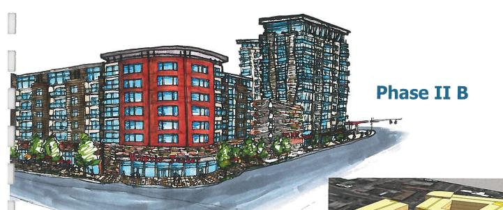
Phase II design will build on the success of the Phase I, with a continuation of similar design elements, features and themes, however to compensate for the increased scale and added volume, Phase II will feature setbacks created along the midpoints of the design to break up the massing and create a friendly, accessible and engaging hub for the community. The result will be a balancing in a
